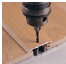
1. Drill hole with a 3 mm drill bit
